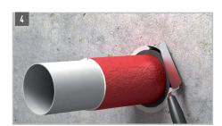
For walls, use one collar on each side. For floors, use one underneath the floor.
