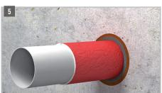
All remaining joints and gaps inside the reveal are to be filled with gypsum or mortar.
