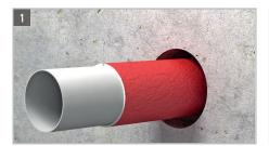
Before the installation of the pipe seal, it is to be checked if all boundary conditions (e.g. type and thickness of wall or floor, type and size of pipes and insulations as well as environmental conditions) comply with the regulations.
