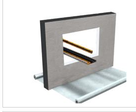
Cable / cable bundles / cable supports accordingly to page 10 with fire protection wrap PYRO-SAFE® DG-CR 1.5 on both sides, length 500 mm and fixation with steel wire.
