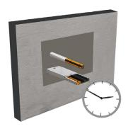
If necessary, cover the floor on both sides with film, clean the recess, wet absorbing surfaces of the recess with water.
