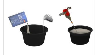
2. Apply the partition compound so that there is a solid, tight connection to the component. Completely fill intermediate spaces and bandage cavities.
