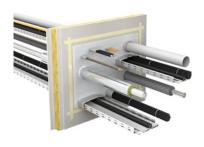
8. Wrap electrical installation conduits and double solar pipes with PYRO-SAFE® DG-CR 1.5 and apply additional protective insulation to non-combustible pipes, multilayer pipes and HVAC split line combinations, if necessary.
