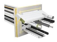
6. Seal the remaining opening / joint gaps with mineral fibre or fill with PYRO-SAFE® FLAMMOTECT-A.
