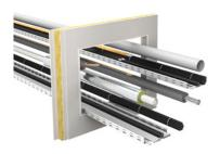
Mask the opening with crepe tape on all sides, keeping 20 mm distance to the edge. Coat the cables with PYRO-SAFE® FLAMMOTECT-A.
