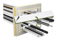
Coat the edges of the mineral fibre boards with PYRO-SAFE® FLAMMOTECT-A and firmly place boards in position.
