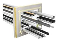
3. Wrap combustible pipes with PYRO-SAFE® DG-CR BS. Wrap multilayer pipes, speedpipes, non-combustible pipes with FEF insulation and HVAC split line combinations with PYRO-SAFE® DG-CR 1.5.
