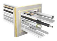
4. Cut mineral fibre boards to size (make cut-outs for the installations).
