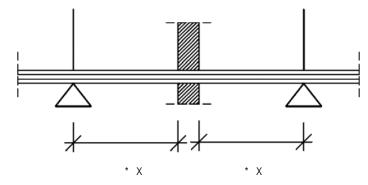
Initial brackets (supports) of the installations in front of the wall penetration sealing system must be made of steel or equivalent material.
