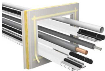
3. Wrap combustible pipes with PYRO-SAFE® DG-CR BS according to page 37.
