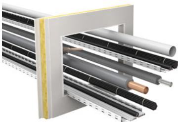
2. Mask the opening with crepe tape on all sides, keeping 20 mm distance to the edge. Coat the cables with PYRO-SAFE® FLAMMOTECT-A; alternatively apply fire protection wrap.
