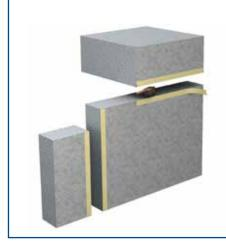
3. Coat one side of the mineral-fibre board with **PYRO-SAFE FLAMMOPLAST KS 1.**
