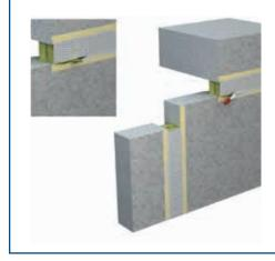
Coat the entire surface of the mineral-fibre board strips with PYRO-SAFE FLAMMOPLAST KS 1 (dry coat thickness ≥ 1.0 mm).
