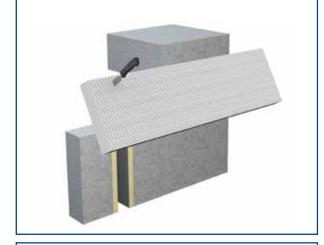
6. Coat the cut edges of the mineral-fibre board strips with PYRO-SAFE FLAMMOPLAST KS 1.
