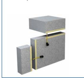
4. Cut the coated mineral-fibre board to a size that is required for the measured joint dimensions.
