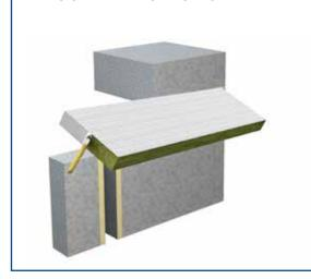
5. Apply PYRO-SAFE FLAMMOPLAST KS 1 to the inside surface of the joint in the region of the mineral-fibre boards, so a covering coat is produced.
