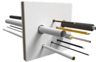
3. Seal on both sides with PYRO-SAFE<sup>®</sup> DG-SC at a depth of 25 mm (20 mm in shaft walls).
